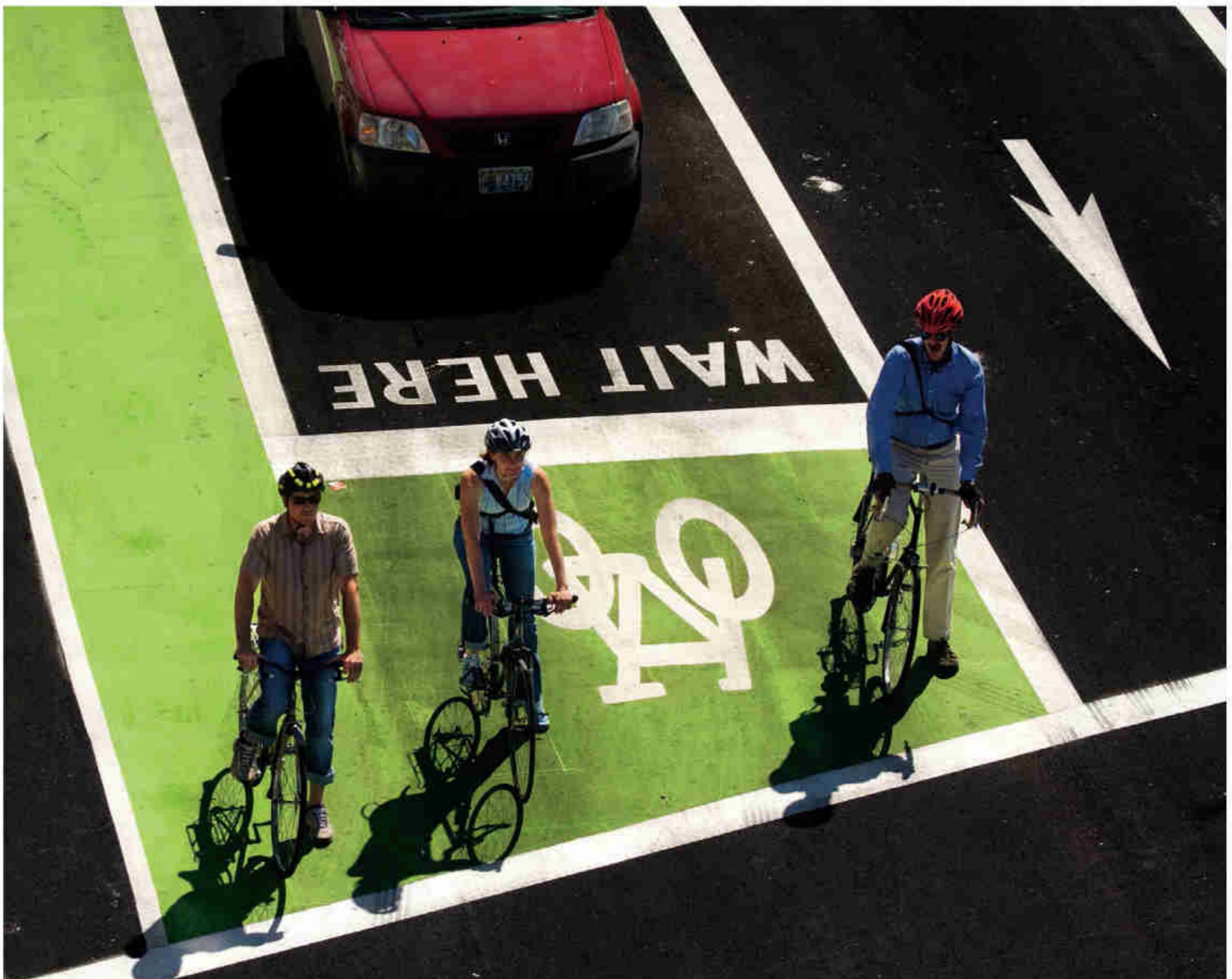
The bike box, a European innovation, gives Portland, Oregon, bikers a jump on traffic.
